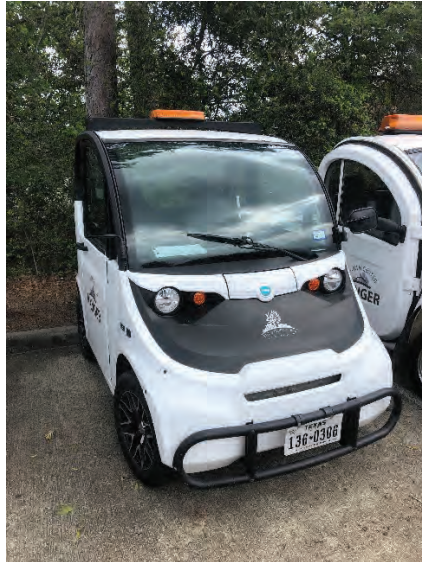
Above: GEM #7, front and rear: note missing passenger side mirror.
