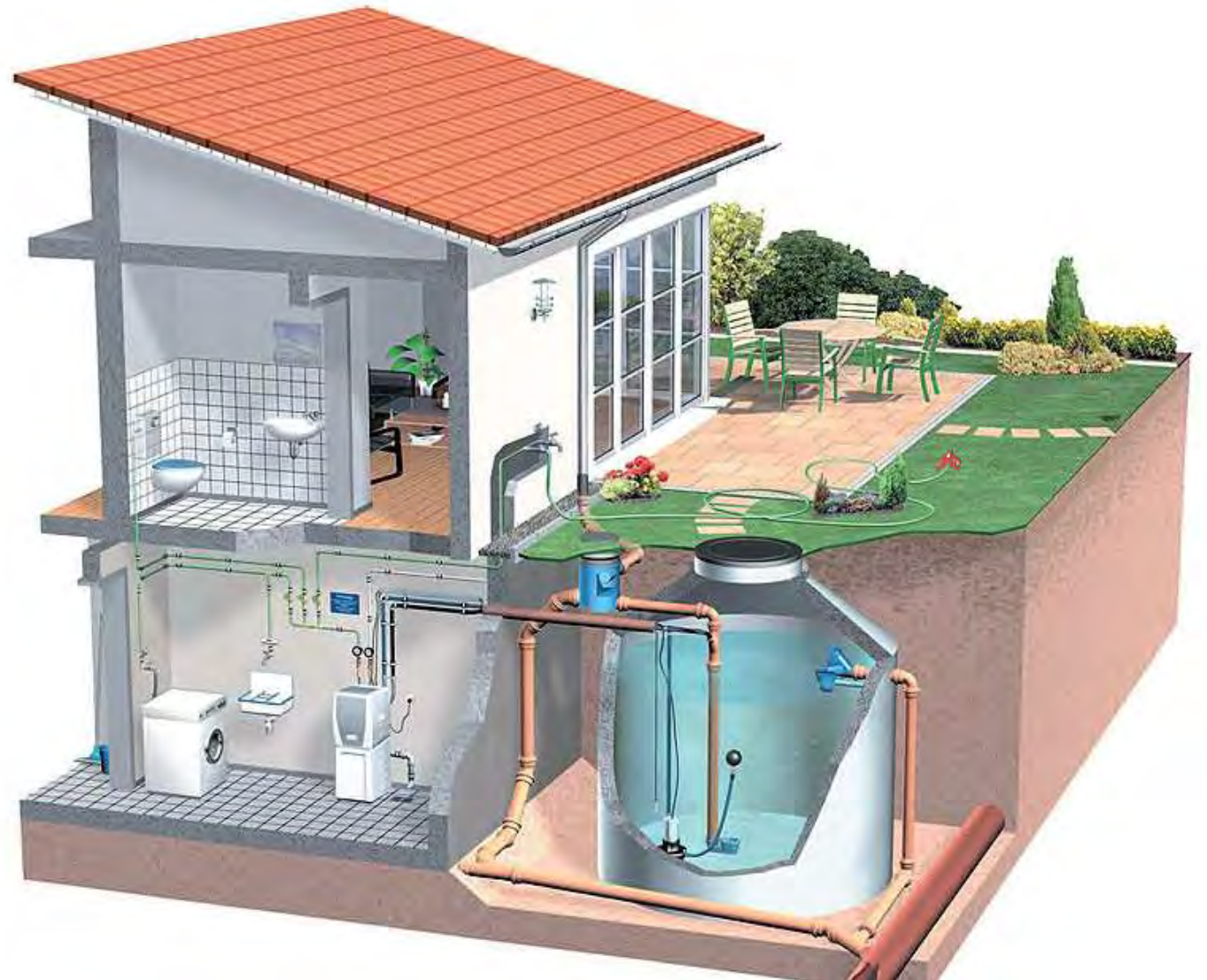
A complete rainwater harvesting system with first-flow filtration, underground cistern and irrigation connections. These systems can be installed with no visible intrusion in the landscape.
